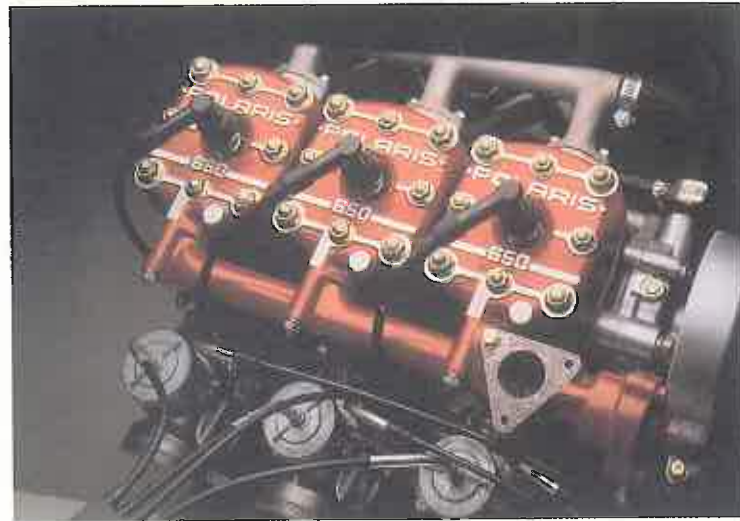
FIGURE 16-21 One of the more popular applications for the two-cycle, loop scavenging-type engine is in a snowmobile. This is a three-cylinder, two-cycle engine. Courtesy of Polaris Industries L.P.
